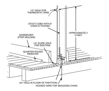
Figure 1. Routing Thermostat Wires
